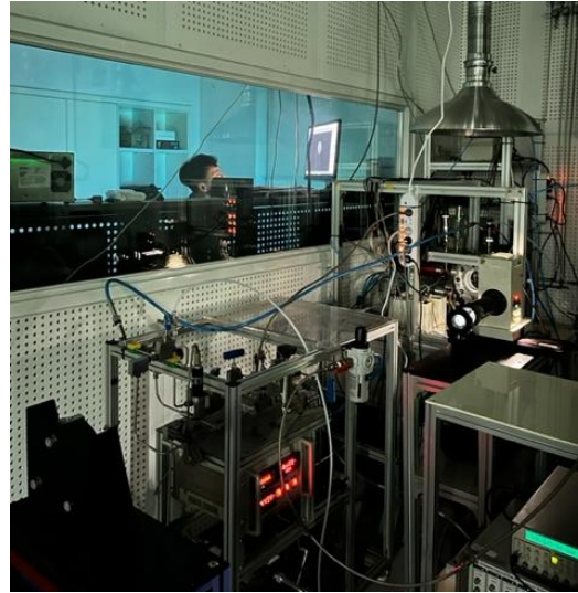
Constant Volume Chamber – fuel characteristics
